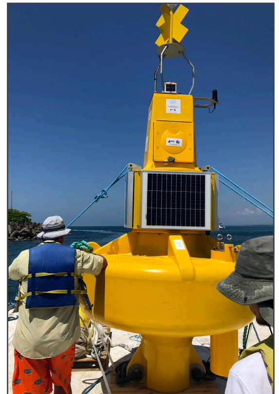
Onsite Field Service and deployment of Hydromet MOTUS Wave Buoy
